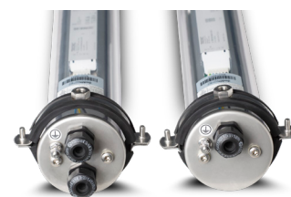
At the end of luminaire can be placed up to two cable glands for easier cable management.
