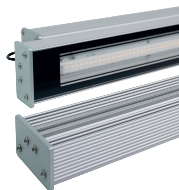
A specially designed aluminium body ensures efficient heat conduction during the warm summer months. On the contrary, a unique front-screen heating system is automatically activated if the luminaire is covered by ice, frost or snow.
